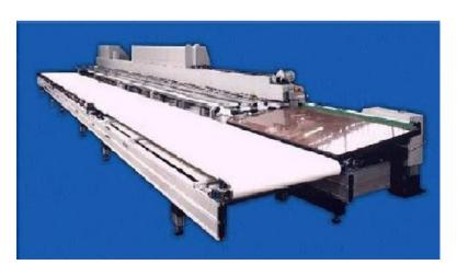
In a little space, PAN RP VT allows the longitudinal panel return to the operator, both when longitudinally or transversally machined on the edge bander. A single operator can control the panel
